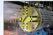
⑤ DO-Jet construction method
